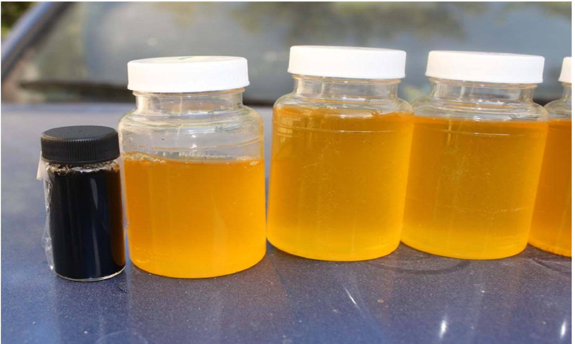
Figure 3. Close-up of samples 1 (left most sample), 2, 3 and partially of sample 4 showing the visual results. Sample 1 was the most contaminated sample from the entire investigation. The black vial represents Hach Pathoscreen with positive results for Sample 1.
